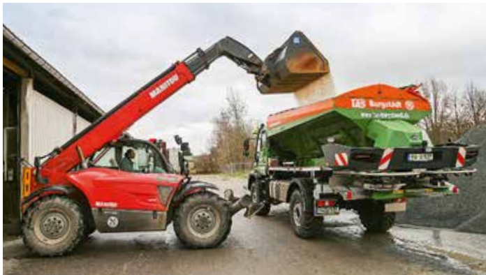
TAS Burgstädt contractors store most of the fertiliser they spread in their own stores. The hopper is filled efficiently by a telehandler.
