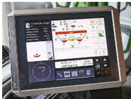
The spreader is operated from the Müller Elektronik terminal in the Unimog cab.
