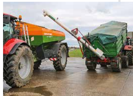
The hopper is auger filled from a trailer parked up at the side of the field.
