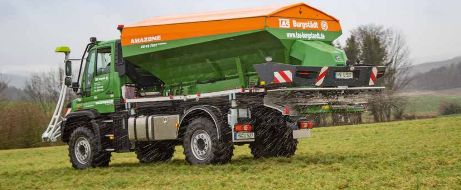
TAS Burgstädt contractors mounted their ZG-TS Truck on a Unimog.
