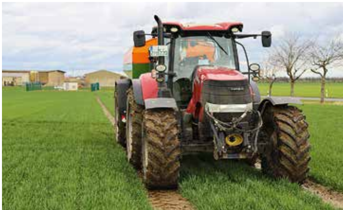
The tramline track width is set by the trailed sprayer at 2.25m.
