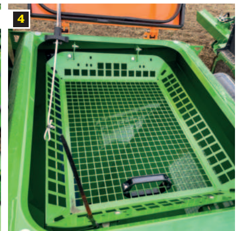
1 The small boxes are an option for the central hopper system. They were a great help for metering small seeds.
