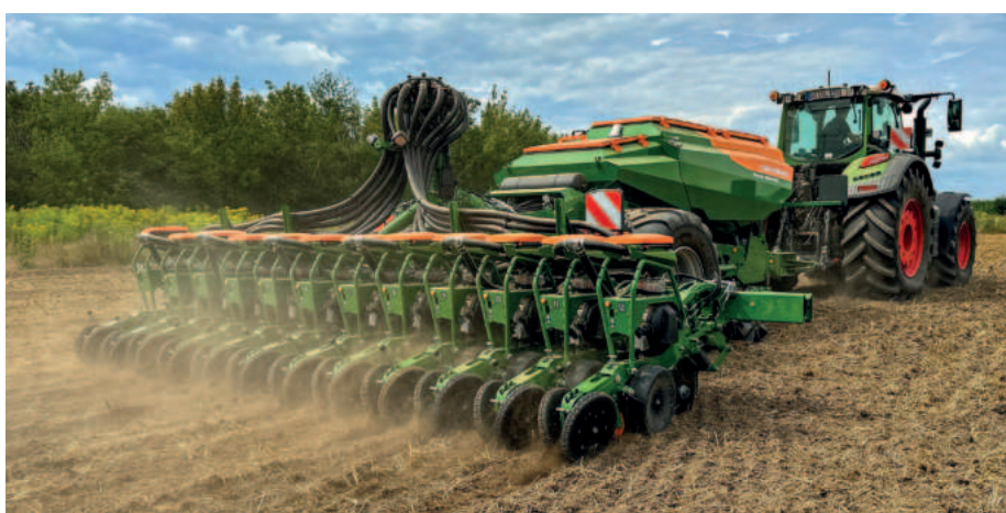
For rapeseed, we used a Precea 6000 TCC with the central seed hopper system. Each row unit was also equipped with the optional 8-litre box.
