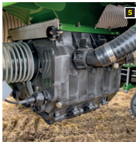
1 The small boxes are an option for the central hopper system. They were a great help for metering small seeds.
