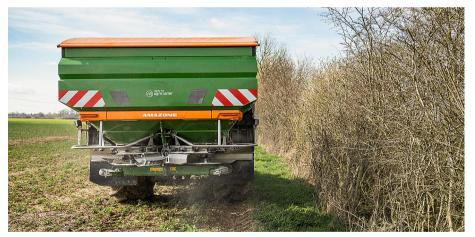
Border TS spreads the full rate all the way up to the border. The system works really well.
