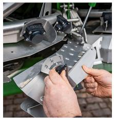
The distance to the boundary can be set on the Border TS deflector (around 1.0-3.0m).
