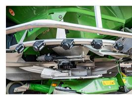
The ArgusTwin radar sensors reliably monitor the machine's spreading pattern.
