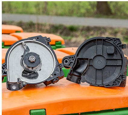
On the left is the housing cover with the portioning arm. Across to the right is an alternative to placing fertilizer in bands.
