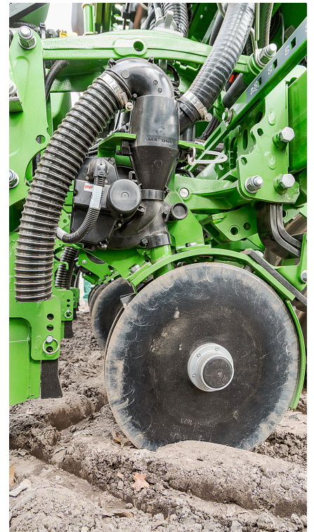
Drills with Fertispot have an additional positioner that's mounted between the air separator and the double-disc coulters.
