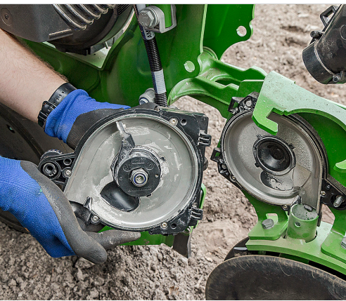
An electric motor in the housing cover drives the Fertispot portioning arms. These arms then inject the granules into the coulters in synch with the seed singling system.
