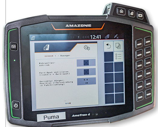
Two additional setting options are added to the in-cab terminal. These activate the fertilizer placement and a correction factor for altering the placement point.
