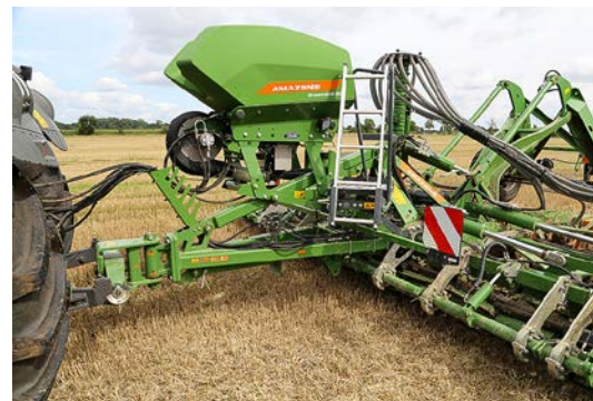
The chunky drawbar is available either as a hydraulic or, as shown here, a rigid version.
