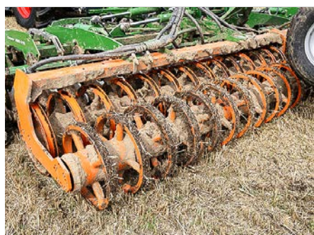
The U-profile rings on the press now have four spokes. There are many press options.
