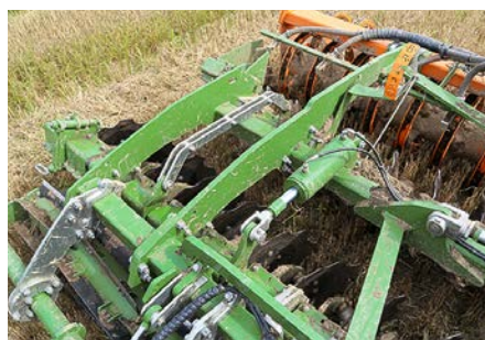
The front and back rows of discs are connected by a mechanical tie rod with depth adjustment done hydraulically – operator-friendly.
