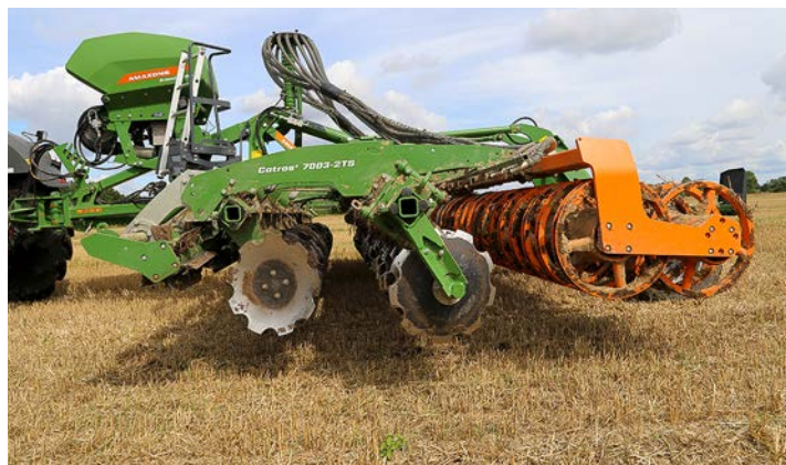
The Smart Frame pivots the two rows of discs to alter the working width while the packer remains fixed.
